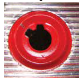
Example showing new notch for headlight switch:
